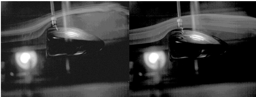
Fig. 4. Smoke visualization over the standard driver head (left) and prototype driver head (right)
